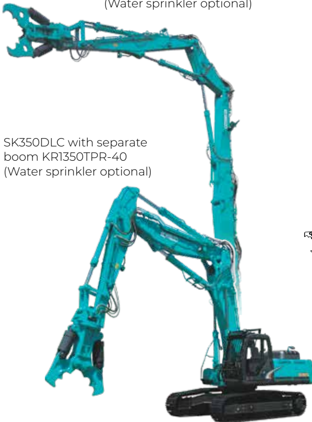
SK350DLC with ultra-long attachment KR1100TPR (Water sprinkler optional)
