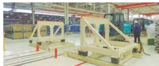
Safety rig for inspection of cabin
