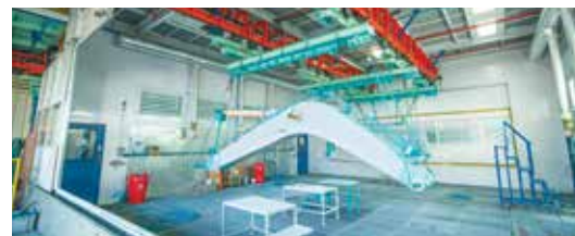
Space saving design for excavator arm paint booth
