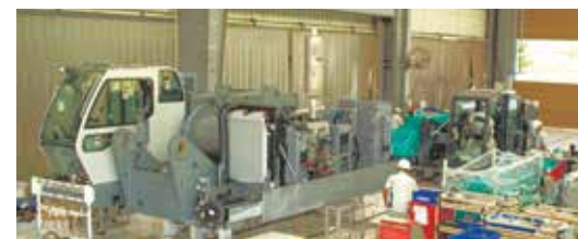
Multi-product assembly line Cranes and Excavators being same assembled in same assembly line
